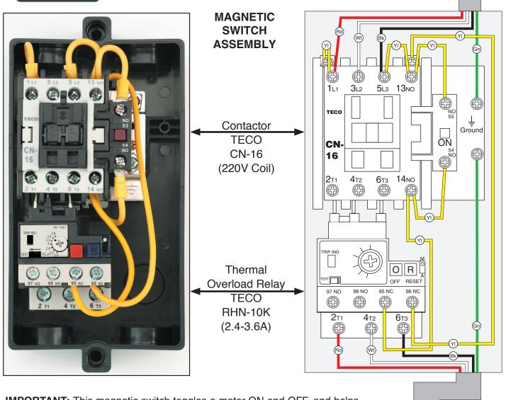
**IMPORTANT:** This magnetic switch toggles a motor ON and OFF, and helps provide thermal overload protection for the motor if operating temperature gradually increases due to heavy work loads. The thermal overload relay inside is not designed to cut power in the event of a sudden motor overload or stall.
